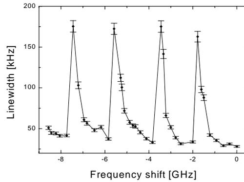
Figure 14. Variations of the linewidth of an ECL measured over a range of external-cavity modes.
