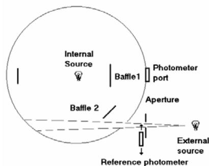
*Figure 3 Set-up for the luminous flux measurement using the absolute integrating sphere method.*
