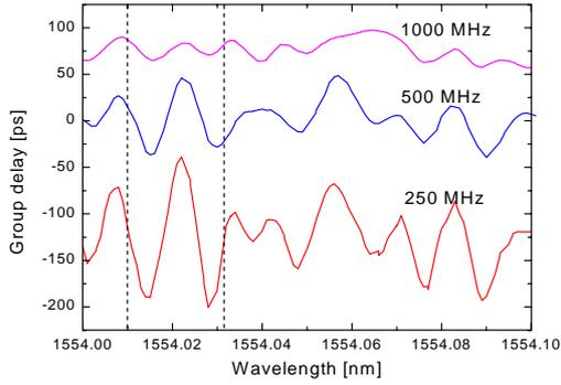
Figure 9. Group delay measured for three different modulation frequencies.
