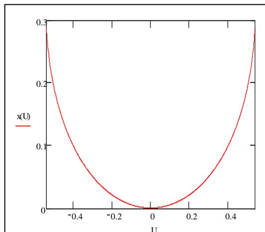
Figure 25. Displacement as a function of DC-bias voltage.
