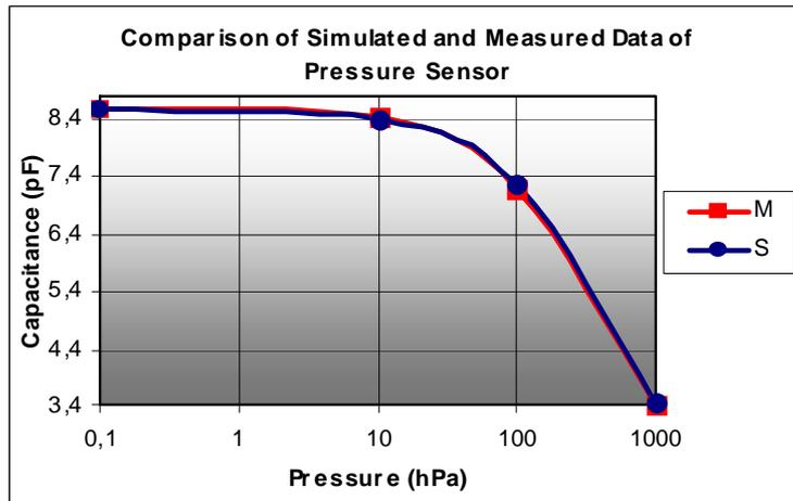
Figure 24. Simulated and measured capacitances as a function of pressure.
