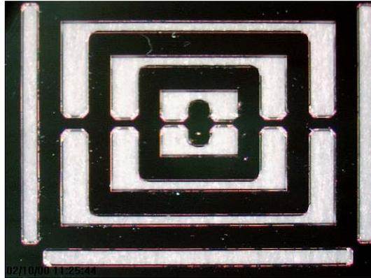
*Figure 20. An example of a torsional, high-Q oscillator structure made with double-sided etching.*
