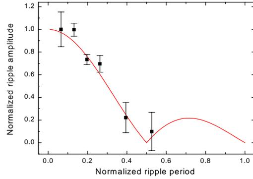
Figure 10. Comparison between the measured and estimated ripple amplitudes.
