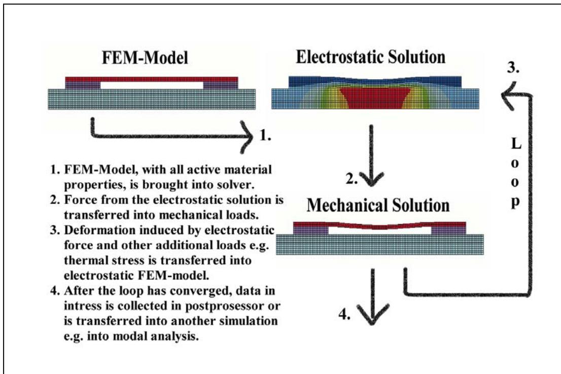
Figure 21. Iterative calculation of electromechanical problem.
