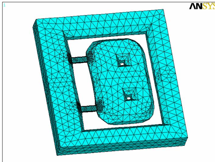
Figure 22. Finite element mesh model of the accelerometer manufactured by VTI Hamlin.
