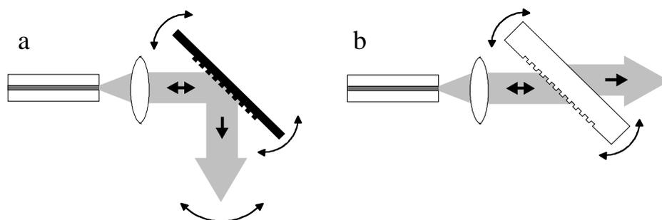
*Figure 6. External-cavity lasers. The traditional reflection geometry (a) and the novel transmission geometry (b). Note that in (b) the output beam direction does not change.*
