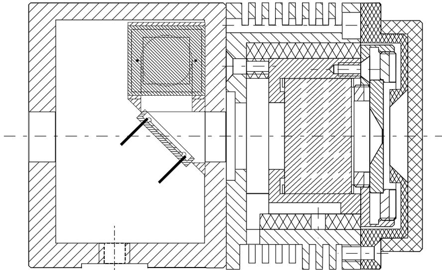
*Figure 2. Cross-sectional view of the trap-based filter radiometer designed and constructed at HUT.*
