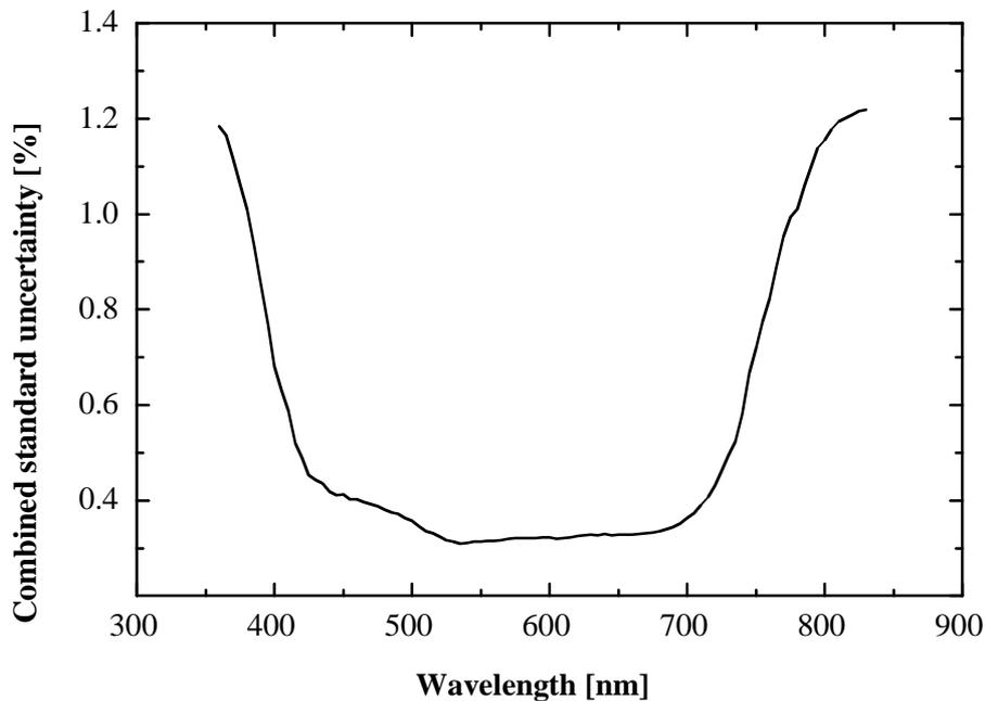
*Figure 4. Combined standard uncertainty of the unit of spectral radiance as a function of wavelength.*
