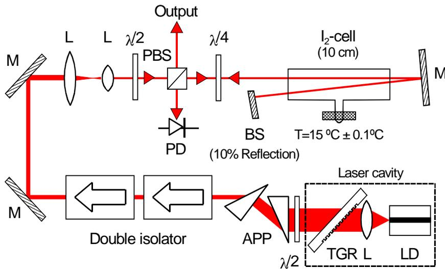
Figure 8. Experimental setup. (LD = laser diode, L = lens, TGR = transmission grating,  $\lambda/2$  = half-wave plate, APP = anamorphic prism pair, M = mirror, PBS = polarising beamsplitter,  $\lambda/4$  = quarter-wave plate, BS = beamsplitter, and PD = photodiode.)
