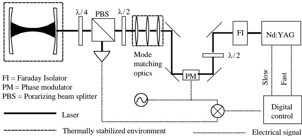
Figure 27. Nd:YAG laser is locked to a high- $Q$  optical resonator using a phase modulation scheme.
