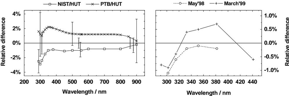
Figure 1. Results of intercomparison measurements and the reproducibility of the realisation of spectral irradiance scale at HUT. Relative differences between the spectral irradiance values a) measured by HUT and given by NIST (empty squares) and by PTB (crosses), bars indicate the level of measurement uncertainties ( $k=2$ ); b) given by NIST and those of obtained from the measurement results in May 1998 (empty circles) and in March 1999 (plus signs) by using the lamp F-434.
