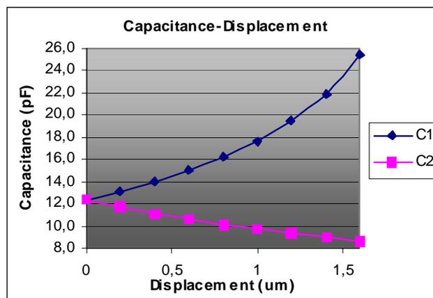
Figure 23. Capacitance as a function of displacement.
