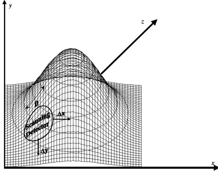
Figure 28. Measurement scheme of the intensity profile of an optical beam. The grid represents the scanning resolution set by  $\Delta x$  and  $\Delta y$ . Grid nodal points are the detector centre positions in individual measurements.
