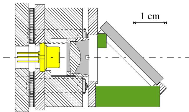
*Figure 7. Mechanical structure of the external-cavity laser based on a transmission grating.*
