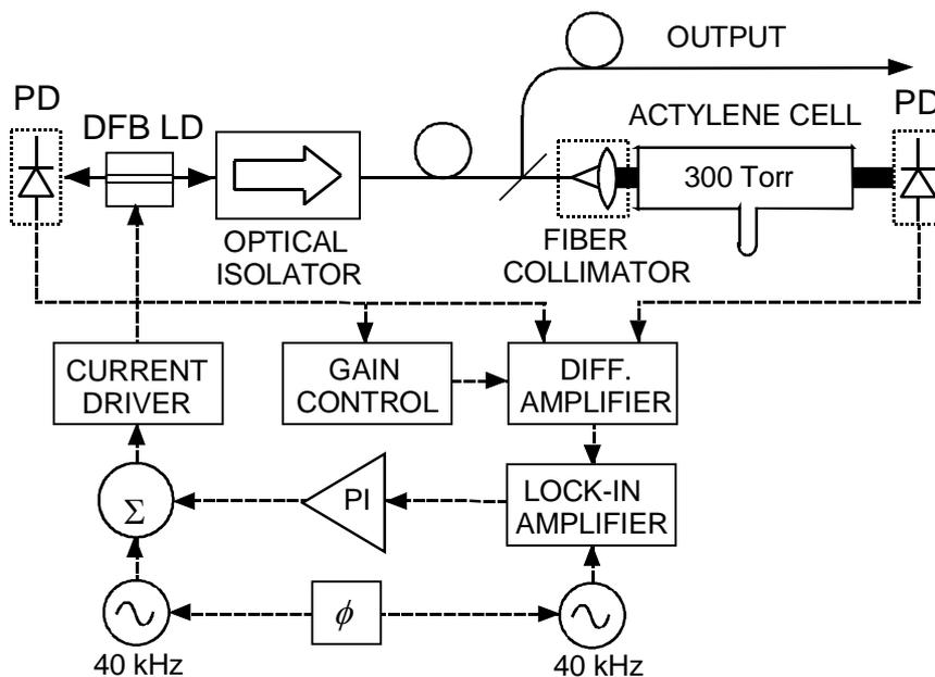
Figure 17. Experimental setup for frequency stabilization.
