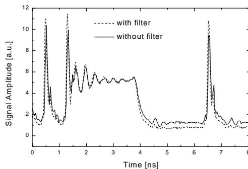
Figure 15. Signals with and without the filter after 350 km of fibre.
