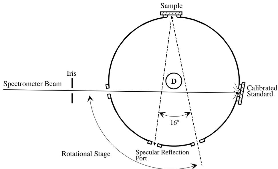
*Figure 5. Top view of the averaging sphere in the setup for measurement of spectral diffuse reflectance. (D: Silicon detector on sphere wall). Interchangeable sample and reference holders can also be used at 8 degrees to achieve 0°/diffuse degrees geometry.*
