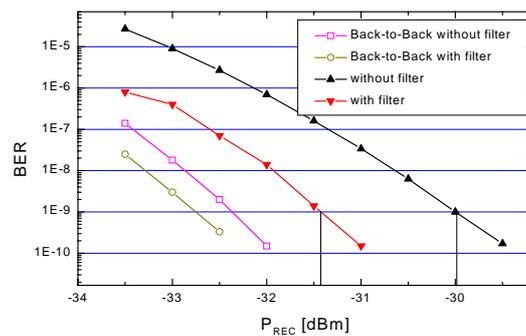
Figure 16. BER measurements with 350 km of fibre.
