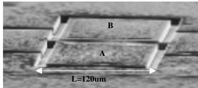
Figure 19. SEM-picture of clamped-clamped beam SOI-resonator.
