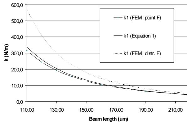
*Figure 18. Spring constant  $k$  of a bridge resonator as the length of the bridge is varied.*
