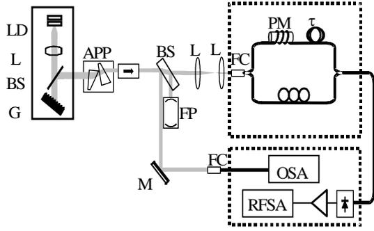
Figure 13. Linewidth measurement setup. G: grating, L: lens, LD: laser diode, APP: anamorphic prisms, BS: beam splitter, M: mirror, FC: fibre collimator, FP: Fabry-Pérot interferometer, OSA: optical spectrum analyzer
