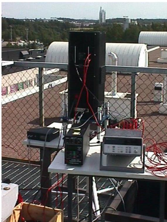
*Figure 5.1.2-1. A photograph of the first prototype calibrator with the associated electronics for lamp control and the monitoring filter radiometers.*
