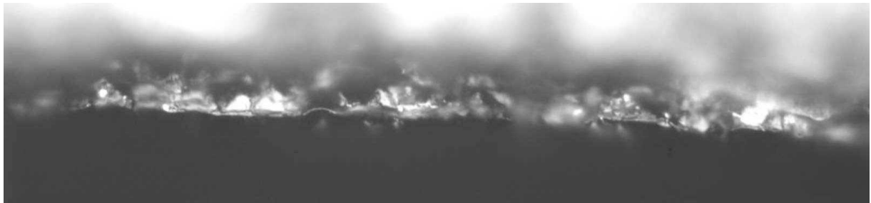
Figure 5.1.4-2. Edge of a precision aperture. The height of the photo corresponds to approximately 40 \mu\text{m} .
