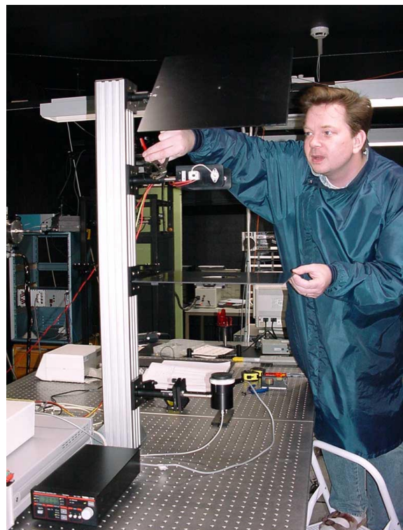
Figure 5.1.7-1. Vertical setup for calibrating DXW-lamps.
