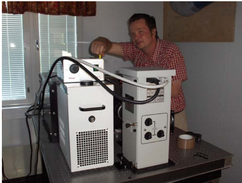
Figure 8. Fine-tuning of the radiator setup in the Observatory of Jokioinen. On the right, one can see the Xe-lamp in its housing and on the left, a water cooler used to circulate the water in the heat absorbing filter.
