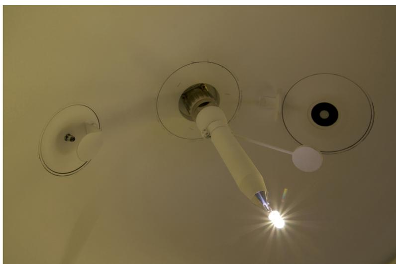
Figure 2. New custom parts of the LED luminous flux sphere.
