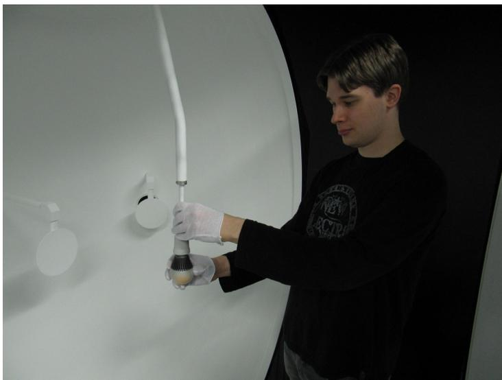
Figure 3. Preparing an LED-lamp for luminous efficacy measurement.
