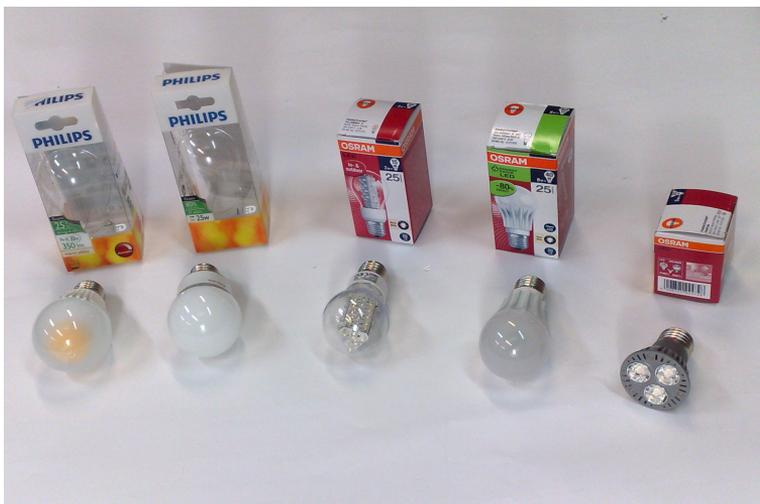
Figure 4. A selection of solid state lamps with E27 base.
