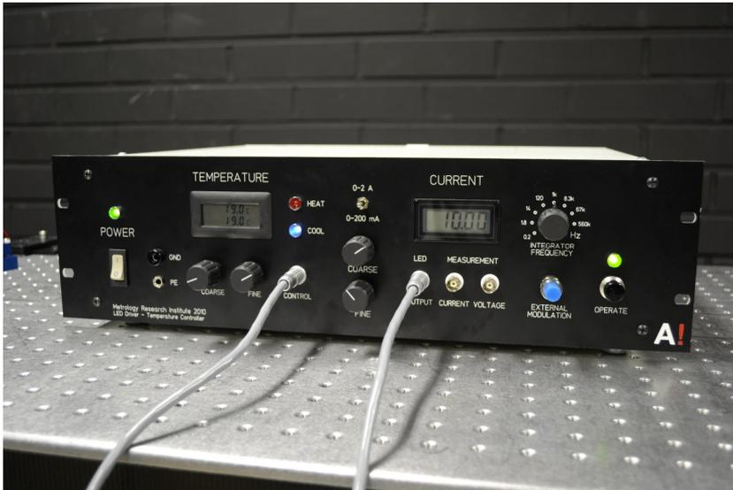
Figure 1. The new LED driver and temperature controller.
