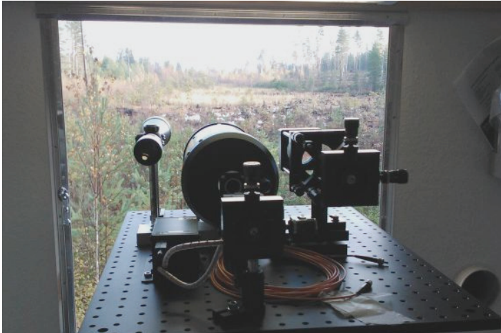
Figure 21. Hyperspectral remote sensing setup in the field tests at the Technical Research Centre of the Finnish Defence Forces.
