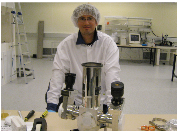
Figure 13. During the low temperature operation, the photodiodes of the PQED are cooled down to 77 K using a liquid nitrogen cryostat.
