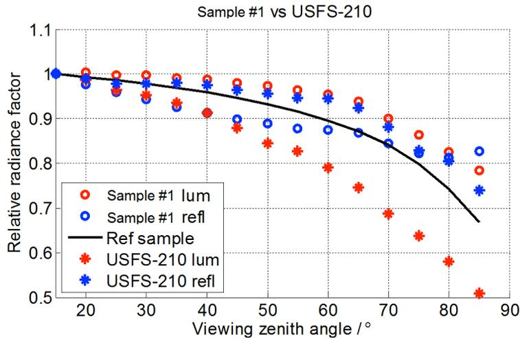
Figure 10. The angular emission of fluorescence from a widely used commercial standard material (USFS-210) and a novel standard material (Sample #1). It can be seen, that the fluorescence emission is more Lambertian for the novel standard material.
