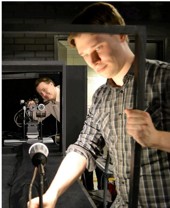
Figure 21. Comparison measurement of LED light sources using the new PQED method and a conventional reference photometer.
