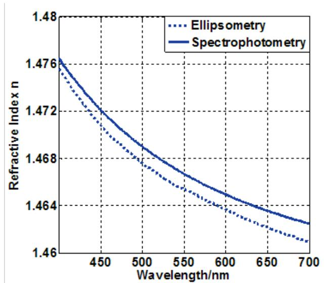
Figure 23. Refractive index of the photodiode's SiO<sub>2</sub> layer as determined by the fitted Cauchy dispersion relation (solid line) and comparison with reported ellipsometry data (dashed line).
