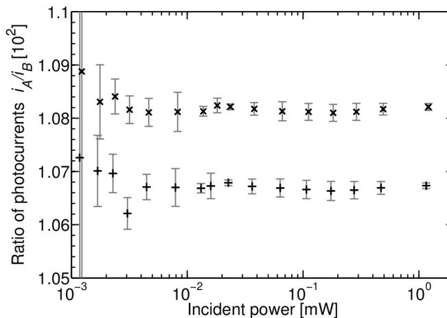
Figure 25. The ratio of photocurrents from the photodiodes mounted inside the attenuator. The signal from photodiode A divided by the signal from photodiode B.
