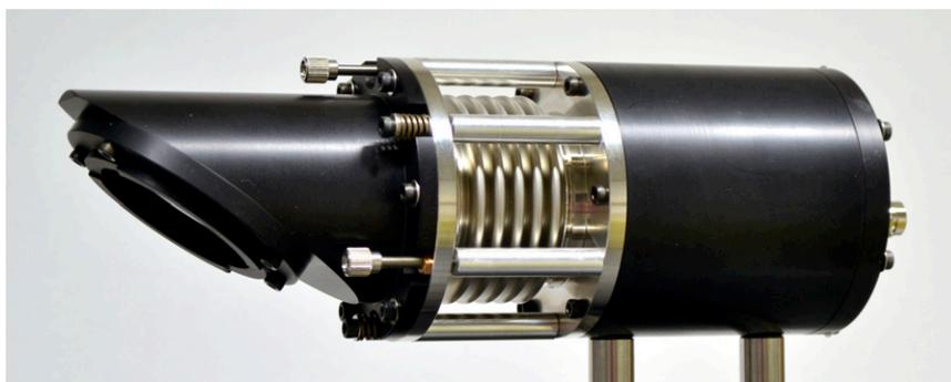
Figure 19. Photograph of the developed room-temperature PQED.
