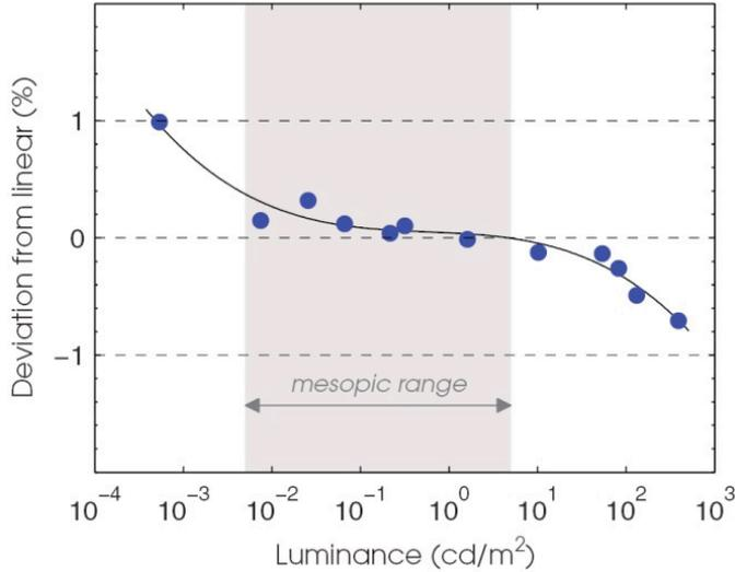
Figure 15. Deviation from the linear response of the developed photopic-scotopic luminance meter as a function of measured photopic luminance.
