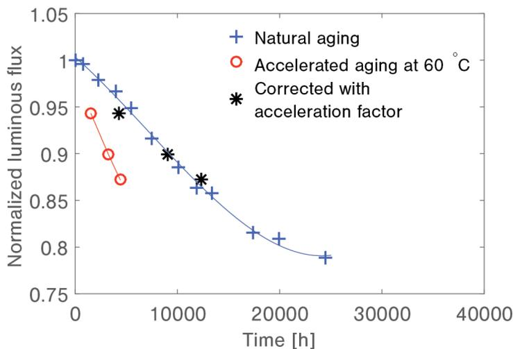
Figure 17. Normalized luminous flux data for Osram A60 lamp. Black asterisks (\*) indicate the accelerated data set, where the time values have been multiplied with an acceleration factor.
