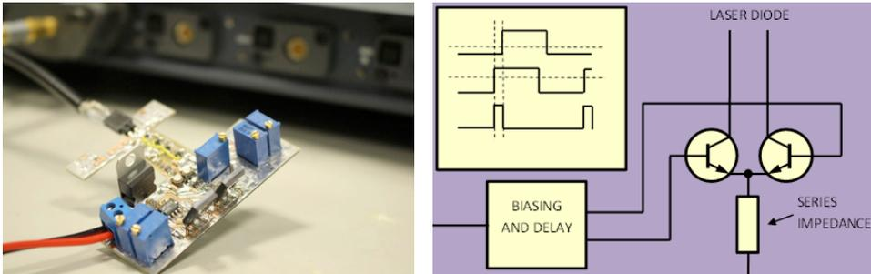
Figure 26. Differential pair driver electronics under testing (left). The basic idea of differential pair driver (right). The current is switched between the dummy load and the laser diode to achieve fast and stable output.
