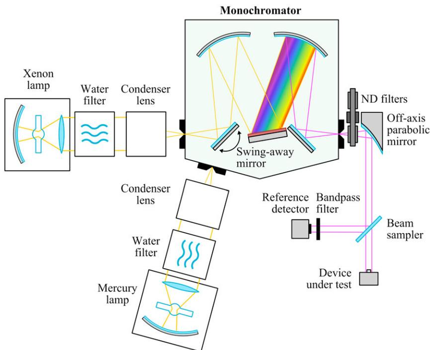
Figure 5: The schematic view of the linearity characterization setup.
