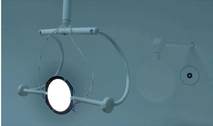
Figure 18. OLED-panel attached for measurement using the developed 2-axis holder.
