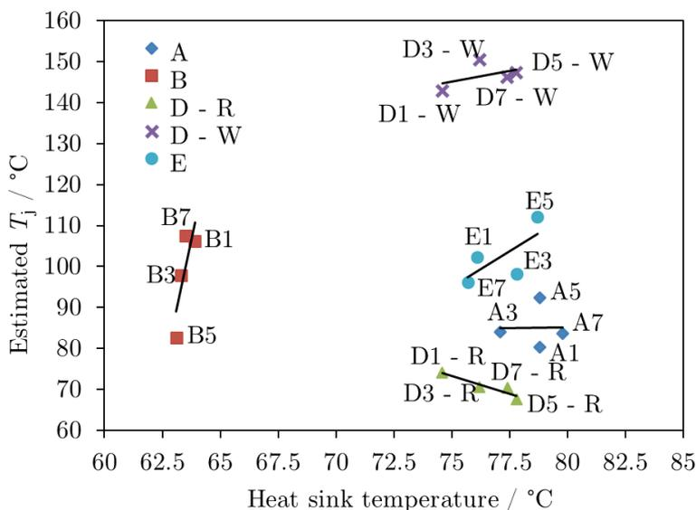
Figure 16. Estimated junction temperatures  $T_j$  of the lamps as a function of the heat sink temperatures.
