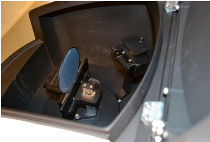
Figure 11. Reflectance measurements of new type of solar cells are carried out by Metrology Research Institute.
