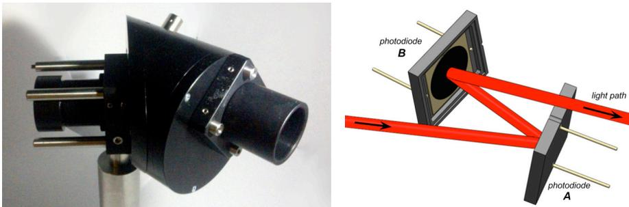
Figure 24. Body and light path of the transmission trap detector–attenuator. Light enters to the leftmost and exits from the rightmost part of the detector.
