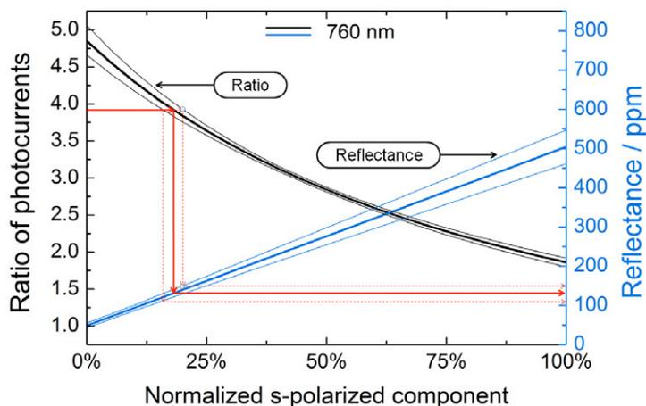
Figure 20. Ratio of photocurrents and corresponding reflectances of the PQED as a function of polarization. Thinner lines indicate the standard uncertainty corridors. Red arrows show the steps to be taken for estimating reflectance based on photocurrent ratio.
