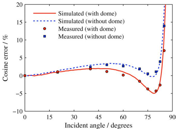
Figure 4: Measured and simulated cosine errors of the diffuser with the fiber connector. The effect of the weather dome of the diffuser assembly on the angular response is clearly visible in the results.
