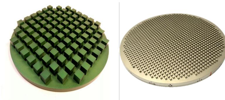
Figure 7. Green anodised aluminium cubes (GAC) target (left) and non-anodised aluminium cubes (NAC) target (right).
