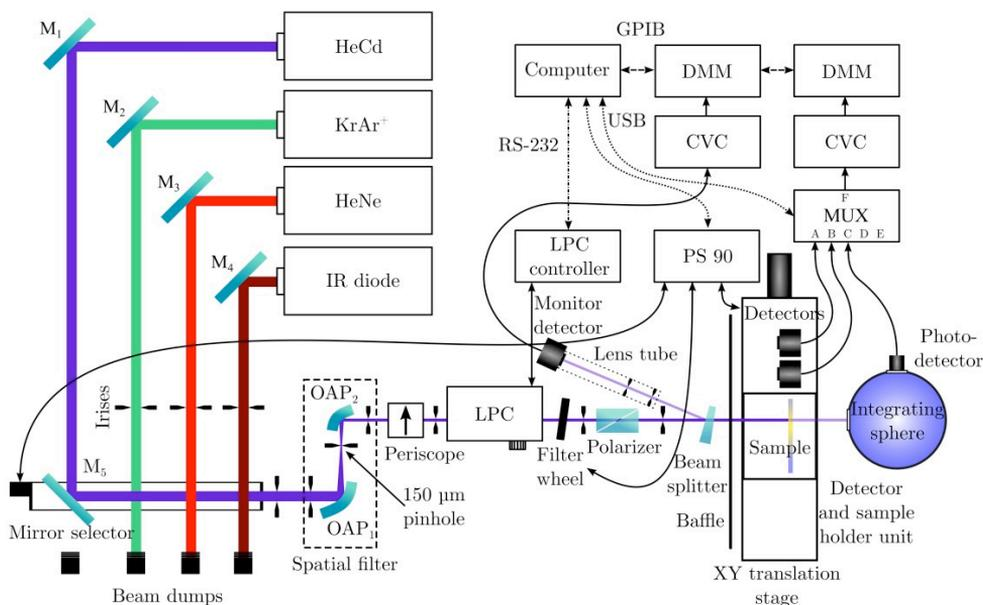
Figure 14. Structure of the laser-based transmittance measurement setup.
