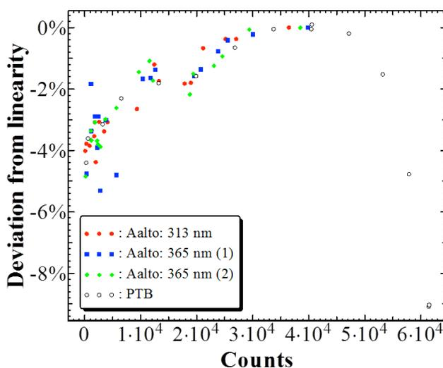
Figure 6: Linearity of AvaSpec spectrometer as a function of instrument counts.
