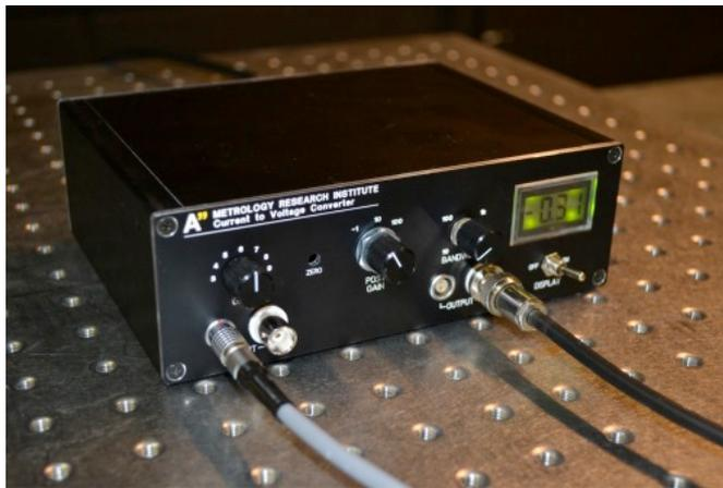
Figure 2. Current-to-voltage converter for measurements with photo detectors developed at the Metrology Research Institute.
