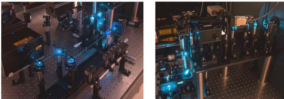
Figure 13. One laser beam is selected by moving the mirror (left), and optics for improving the quality of the selected beam (right).
