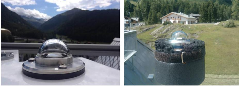
Figure 3: Diffuser of the Brewer spectrophotometer (left), and the fiber-coupled diffuser (right) during the measurement campaign in Davos, Switzerland in July 2014.
