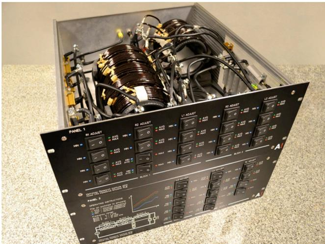
Figure 1. Adjustable power line impedance emulator (APLIE) developed for luminous efficacy measurements of energy-saving lighting products.
