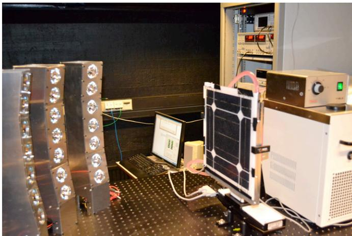
Figure 12. Differential spectral responsivity measurement facility.
