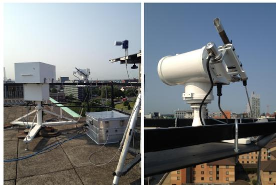
*Figure 1. METCON dual channel spectrometer system deployed at Manchester Surface Radiation Monitoring Site.*
