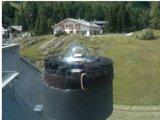
Figure 4. a) Photograph of the new fiber coupled Schreder diffuser b) Measured (symbols) and simulated (lines) cosine errors for the new fiber diffuser. The effect of the quartz dome can be clearly seen by comparing the results with and without the dome.
