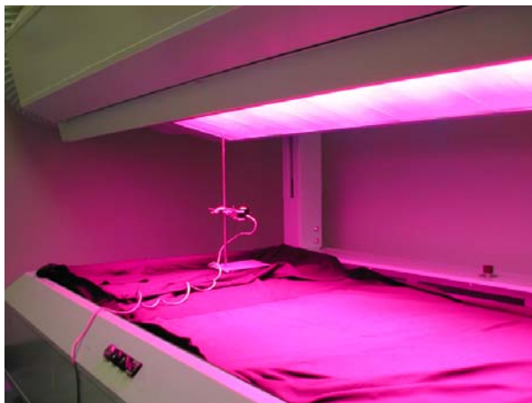
Figure 1. UV mapping of the irradiance over the area normally occupied by the patient. The sheet was used to avoid reflections.
