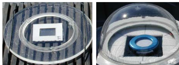
Figure 2. Polysulphone film badge under quartz glass (left), and spore dosimeter under quartz dome (right) on SSI's roof.
