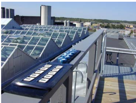
Figure 4. Ten polysulphone film badges (front) and ten bacteria spore dosimeters (behind) exposed to a full day of summer sunshine 4.6.2004 on SSI's roof platform.
