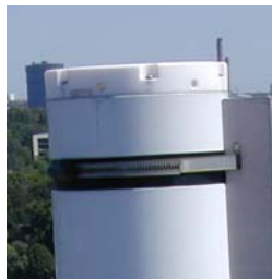
Figure 3. SSI's UV-monitoring instrument is a multichannel UV-radiometer (Biospherical Instr. GUV541) at Solna, Stockholm (59.35°N). It reports the global solar UV-index in six-minute intervals on the SSI-website http://uvindex.ssi.se
