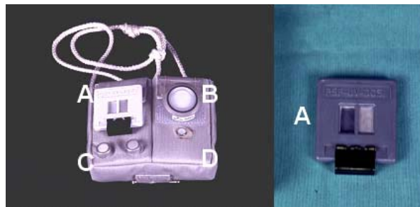
Figure 1. Personal UV dosimeters to measure biological-effective UV radiation (A) Polysulphone film dosimeter (Dermatology/Technische Universität Dresden, Germany) (B) VioSpor dosimeter (Fa. Biosense, Bornheim, Germany) (C) X2000 data logger dosimeter (Fa. Gigahertz-Optik, Puchheim, Germany) (D) UVDAN data logger dosimeter (Fa. ESYS, Berlin / AWI Bremerhaven, Germany).
