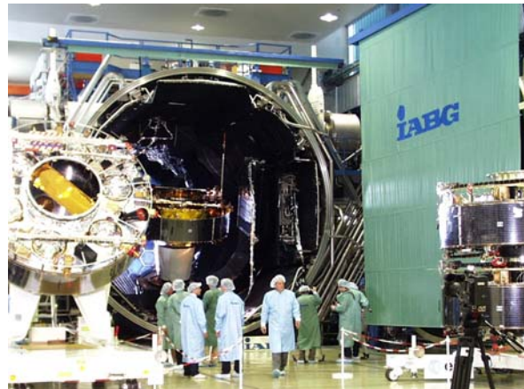
Figure 2. Solar Simulator WSA/TVA at IABG.
