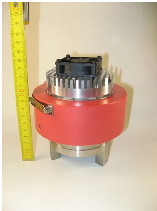
Figure 3. Assembled prototype of the monitoring source based on UV-LEDs.
